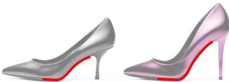
Fig. 19 Shank embedded in outsole-for different heel height – taken from (Lee, 2012)
