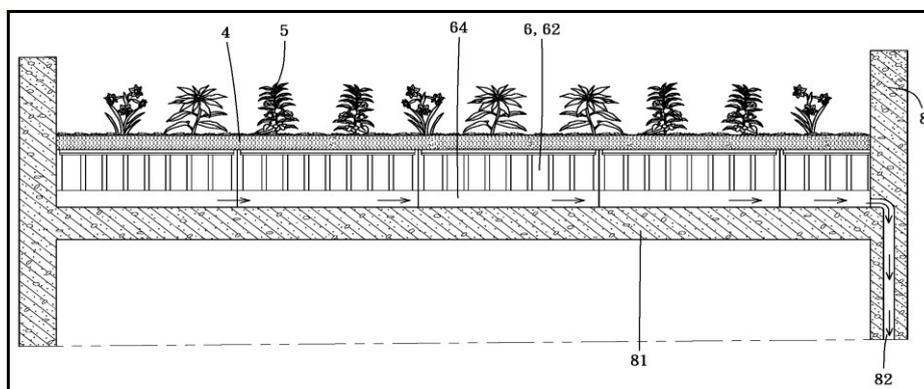
**Figure 8. Type IV: Structure used on rooftop with plants**
