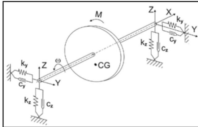
**Figure 3. Three DOF Laval rotor. X, Y, Z – coordinate system,  $c_y, c_z$  – damping coefficients,  $k_y, k_z$  – stiffness coefficients,  $\omega$  – angular velocity,  $M$  – torque, CG – center of gravity**
