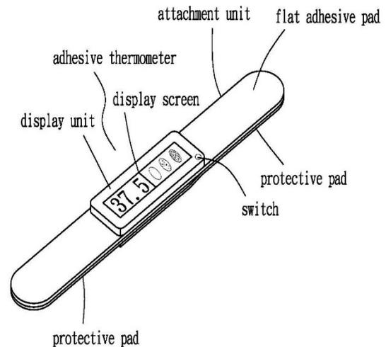
**Fig.6.** Exploded view of Multi-Color Display Adhesive Thermometer
