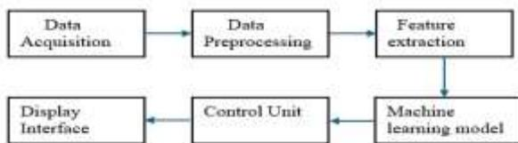
**Fig. 6.** Block diagram for implementing medical image processing with machine learning on a field-programmable gate array.
