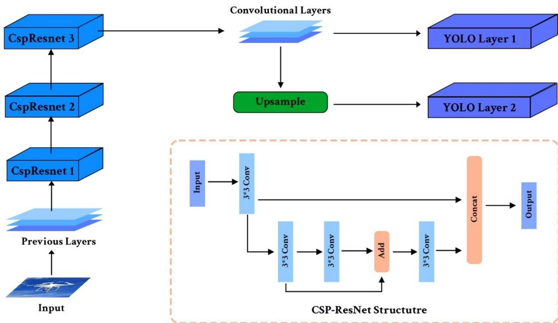
**Fig 1.** Layered Architecture of YOLOv5x
